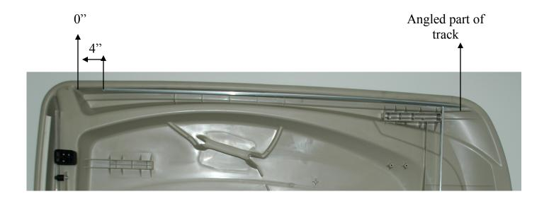
Step 1: Place ruler in corner where diagram reads zero and measure forward 4" and make mark with pencil as shown above on the left. This will give you the placement of the start of the track. Note that the forward end of the track has an angle cut into the flat piece of the track. The flat part of the track will be pointing upward, and the round part of the track will be at the bottom with the slit pointing outward from top.
