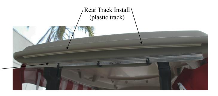
Step 1: Using plastic track, (flat piece of track will be pointing upward, and round part of the track will be at the bottom with the slit pointing outward from top) center track across rear of the top.
